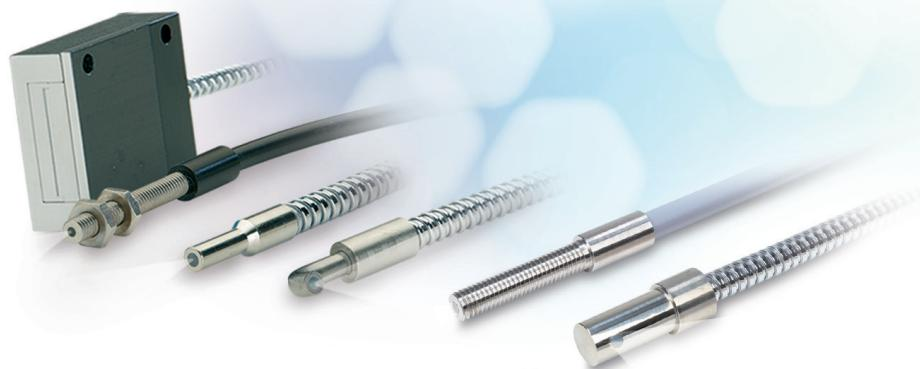
In the case of the reflex sensor, the infrared light emitted by the controller is guided to the detecting object via the sensor's fiber-optic light guides and reflected there. Both diffuse and directly reflected components are present in the back-reflected infrared light. The reflected light components of the object to be detected are received by the same sensor and transmitted back to the controller via the optical fiber for evaluation.
