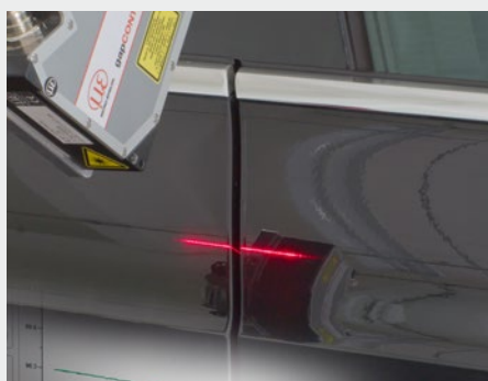
Gap and flushness measurement on bodywork parts
